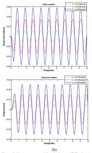
Figure 2: Motion response of the vehicle at v=17.5km/h, (a) bounce motion, (b) Pitch Motion
