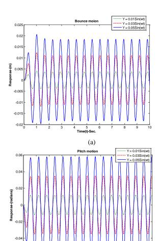
Figure 4: Motion response of the vehicle at v=28.65 km/h, (a) Bounce motion, (b) Pitch Motion
