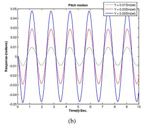
Figure 1: Motion response of the vehicle at v=11.5km/h, (a) bounce motion, (b) Pitch Motion
