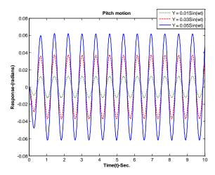
Figure 3: Motion response of the vehicle at v=22.9 km/h, (a) Bounce motion, (b) Pitch Motion
